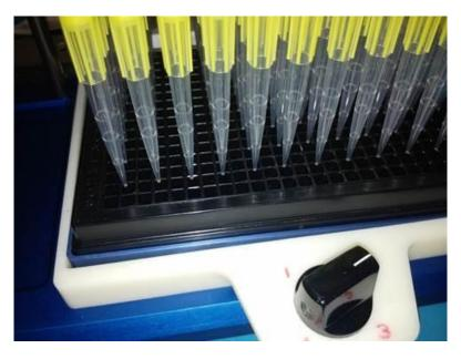
Again rotate the knob to Position #3 and the plate is positioned in the well below. Each position positively clicks in place.
