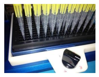
Finally rotate to Position #4 to finish the 96 to 384 dispenses.
