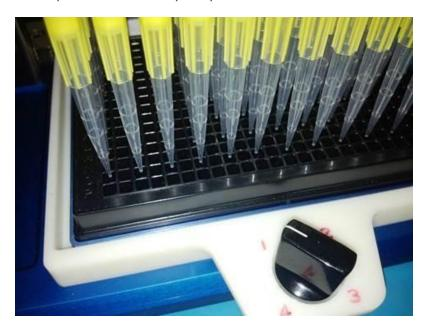
Now rotate the knob to Position #2, the microplate will then move to the adjacent empty well below the 96 channel tips to dispense into. Each position positively clicks in place without needing to align by hand.
