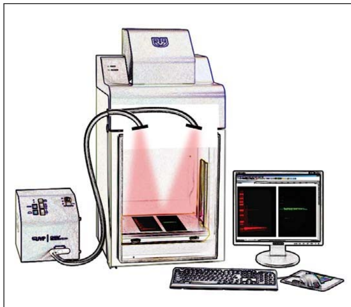
Figure 3. BioSpectrum connected to the BioLite. Together, the BioSpectrum and BioLite are a powerful combination that, depending on the filters used, are able to specifically excite and illuminate at wavelengths from 365 to 765nm and read emissions from 400 to 850nm. UP to 8 excitation and 5 emission wavelengths are possible in a single experiment.
